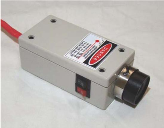
The PL-160 is a class IIIb laser system which includes the biofeedback laser interface, AC power adapter, laser safety glasses, protective case and a fully adjustable single aperture dual laser system. Laser configuration includes 1-650nm and 1-780nm diodes with a total combined output  $\leq 160\text{mW}$ . 50% duty cycle / 2500Hz output frequency.
